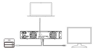
B. DR8-TB3: Let its TB A port connect to Host (PC/Workstation/Server), TB B port to a monitor, and mDP port to the second monitor.
